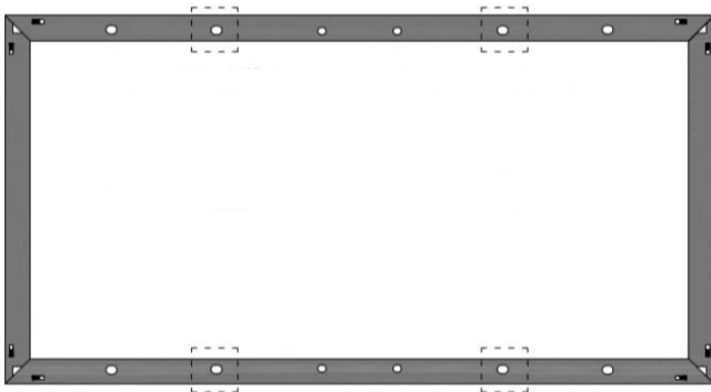
Figure 1.2 : Bolt mounting (4 mounting holes)
